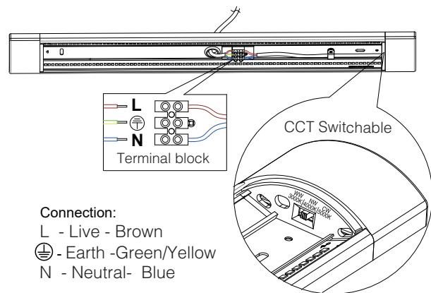
Step 3: Individually connect the Live wire, Neutral wire and Earth wire into the terminal block.
