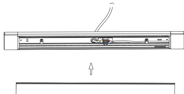
Step 4: Assemble LED diffuser back to base housing.
