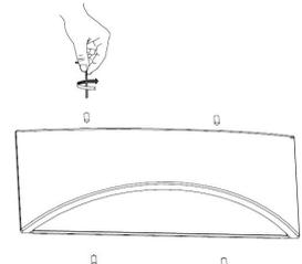
Attach fitting back onto the bracket by fastening the two fixing screws.
