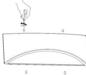
Unscrew and remove mounting bracket by the allen key supplied.
