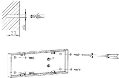
Mount the bracket on the desired surface using the two screws supplied.
