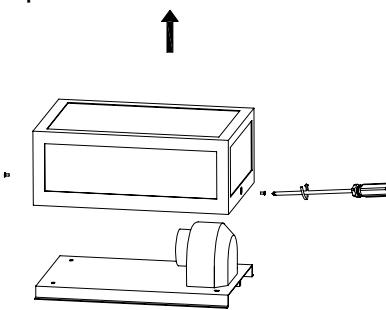
Unscrew and remove the mounting bracket using the allen key supplied.
