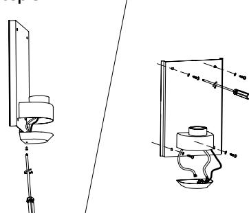
Mount the bracket on the desired surface using the screws supplied.
