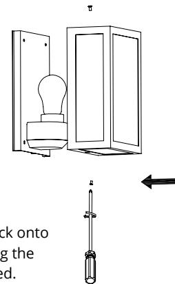
Attach fitting back onto the bracket using the allen key supplied.
