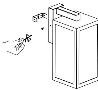
Unscrew and remove the mounting bracket using the allen key supplied.
