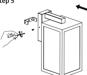
Attach fitting back onto the bracket using the allen key supplied.
