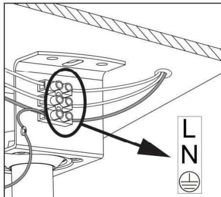
Fix the Earth cable and complete all electrical connections at the mounting bracket.
