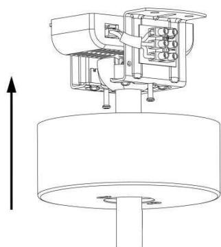
Slide the canopy upward onto the mounting bracket and rotate it counter-clockwise to lock it in place. Check if both mounting bracket tabs are fully engaged within the canopy slots. The canopy should have an approximate 3mm gap from the ceiling.
