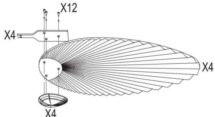
Install the blade holder the bottom of the motor using the retained screws from the plastic inserts. Tighten and secure blade bracket with screw and washer provided. Repeat this procedure until all the blade holders installed.
