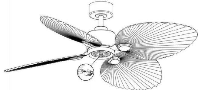
Plug the plug from light kit into the plug the fan.
