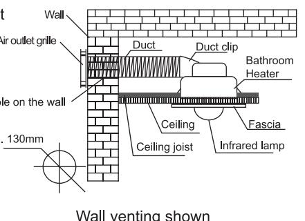
**Note:** Since the length of each duct is 1.5m, make sure that from the centre of installation position there should be a distance within 1.5m to the outside vent.
