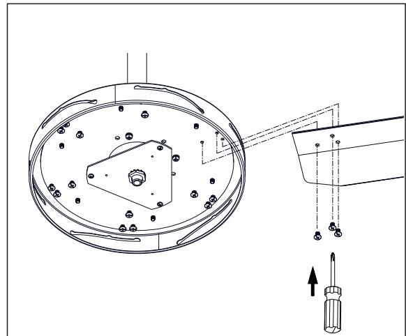
Install the blades to the bottom of the motor. Tighten and secure blade with screw and washer provided. Repeat this procedure until all blades are installed.
