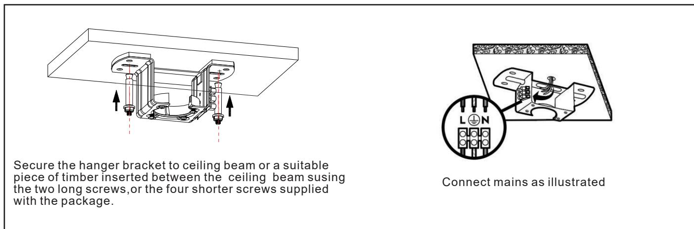
Secure the hanger bracket to ceiling beam or a suitable piece of timber inserted between the ceiling beam using the two long screws, or the four shorter screws supplied with the package.
