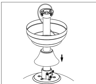
Loosen two set screws on the downrod support and then place downrod into the downrod support. Align the Clevis Pin holes in the Downrod with the holes in the Downrod support. Be sure to push the straight leg of the Hairpin Clip through the hole near the end of the Clevis Pin until the curved portion of the Hairpin snaps around the Clevis Pin. Finally, re-tighten the two set screws.
