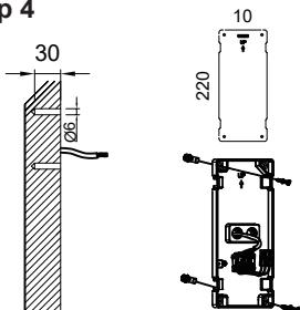
Fit main cable and the silicon cover through the entry at the back.
