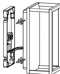
Remove mounting bracket by the Allen Key.
