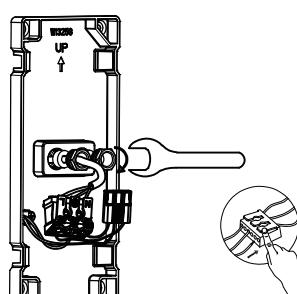
Drill holes and mount the bracket on desired surface.
