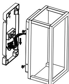
Attach fitting back onto the bracket by fastening the two fixing screws.
