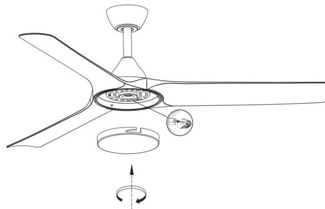
Align with the gap on the LED mounting plate and press down firmly while twisting on.
