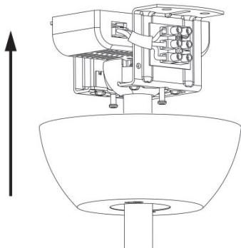
Slide the canopy upward onto the mounting bracket and rotate it counter-clockwise to lock it in place. Check if both mounting bracket tabs are fully engaged within the canopy slots. The canopy should have an approximate 3mm gap from the ceiling.
